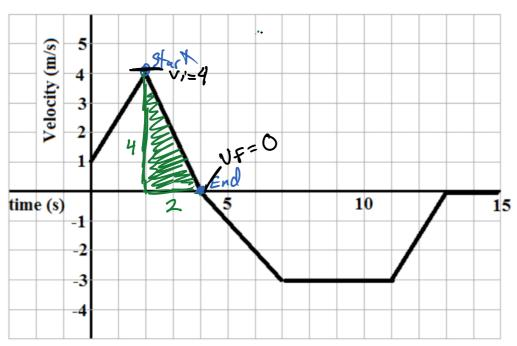
To find the displacement from a Velocity-Time Graph you would find the average velocity then multiply that by the amount of time it travels at that velocity. Vary = Vi+Vf
